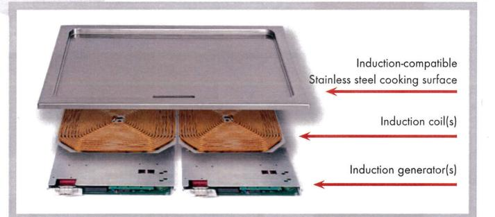
Berner induction griddles are renowned for maximum energy efficiency. The short heat-up time due to induction power enables energy to be saved. It only takes a matter of minutes to reach cooking temperature after switching the appliance on.
